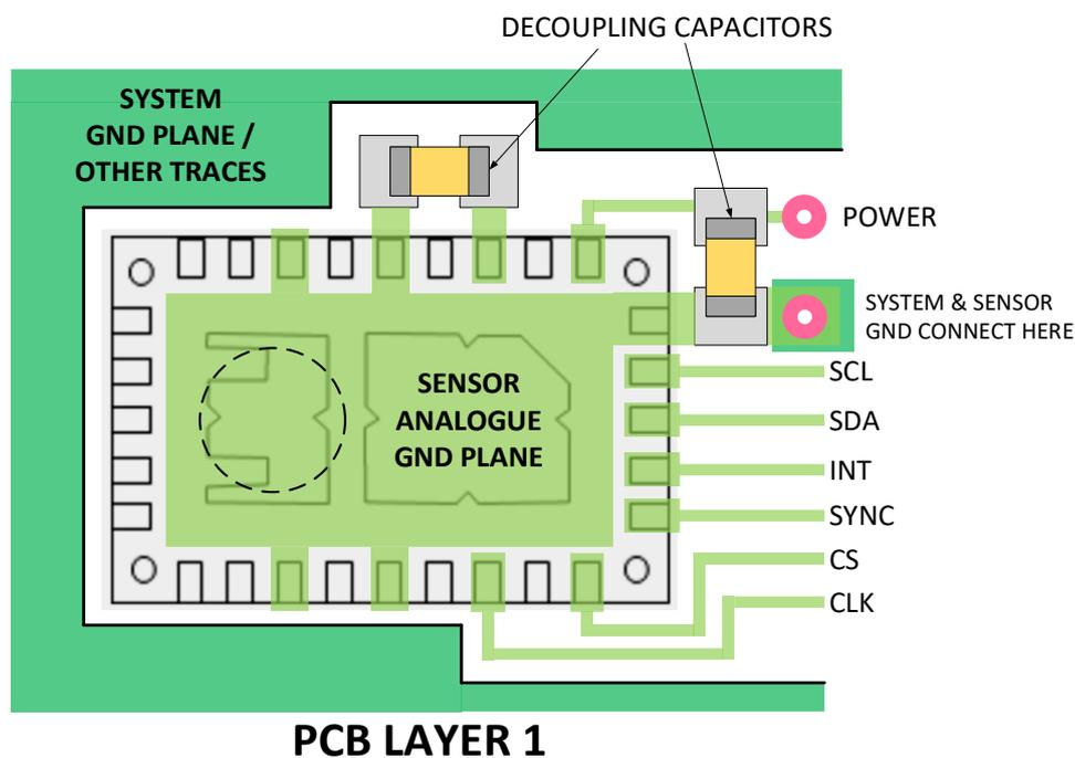
*Figure 2 - Layer 1 PCB layout in the sensor area*
