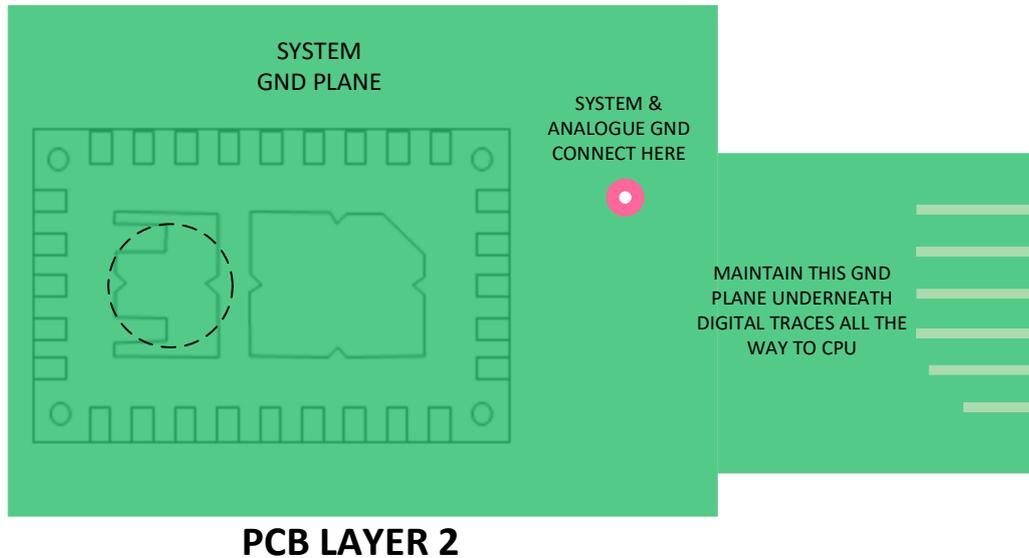
Figure 3 – Layer 2 PCB layout in the sensor area
