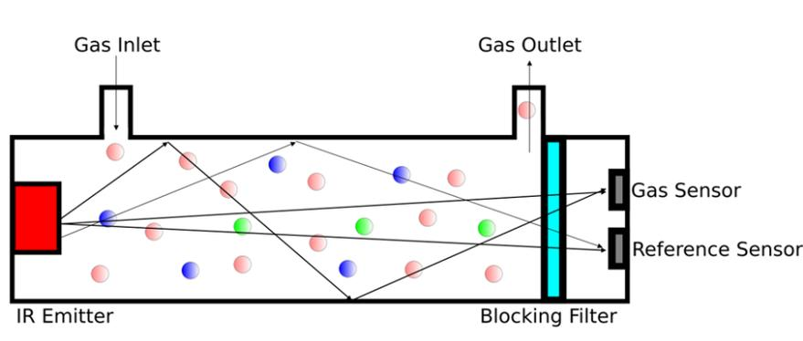
Figure 1 Simplified sketch of an NDIR spectroscopy system
