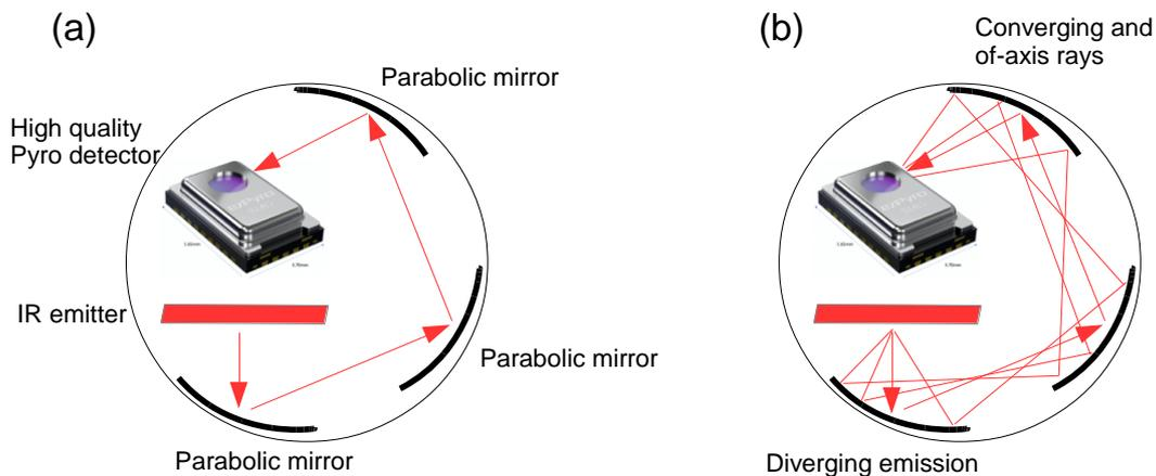
Figure 8 (a) Round gas cell system design (b) diverging IR emission on a pyro detector
