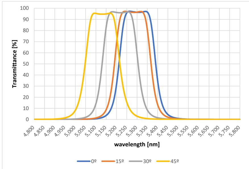
Figure 9 Optical spectrum of a 5.30/180 IR filter under four different angles of incidence
