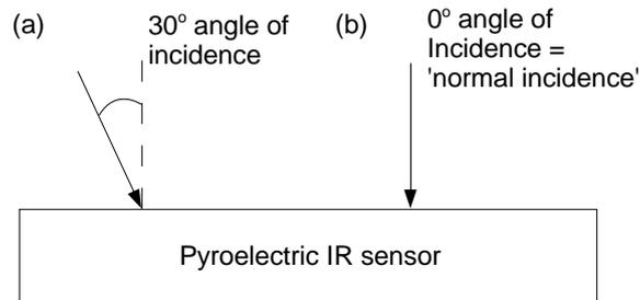
Figure 7 Exemplar light angles of incidence on the detector surface. (a) 30°, (b) 0°, also called 'normal'
