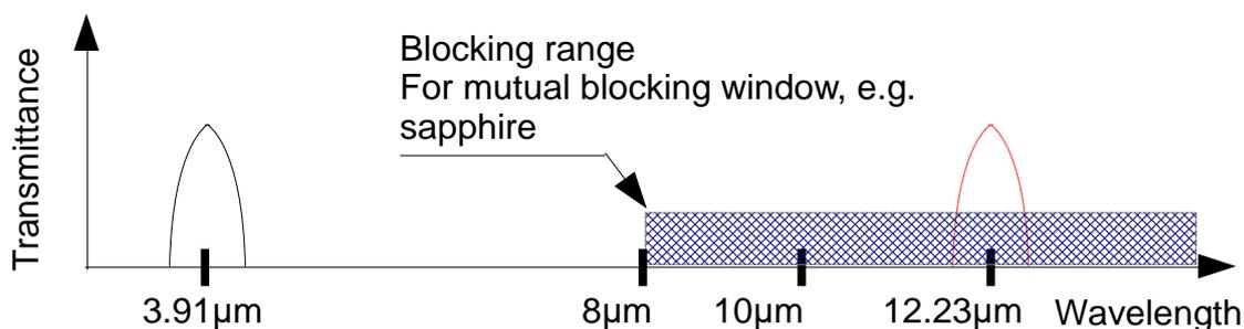
Figure 5 Simplified sketch showing transmittance spectra for both channels blocked with a mutual blocking window
