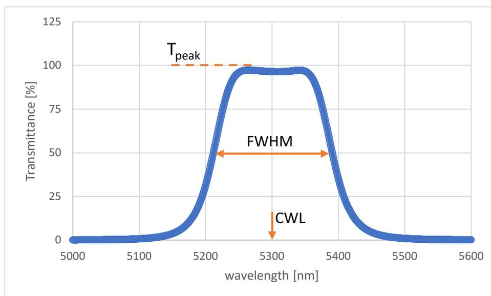
Figure 2 Optical spectrum of a 5.30/180 IR filter
