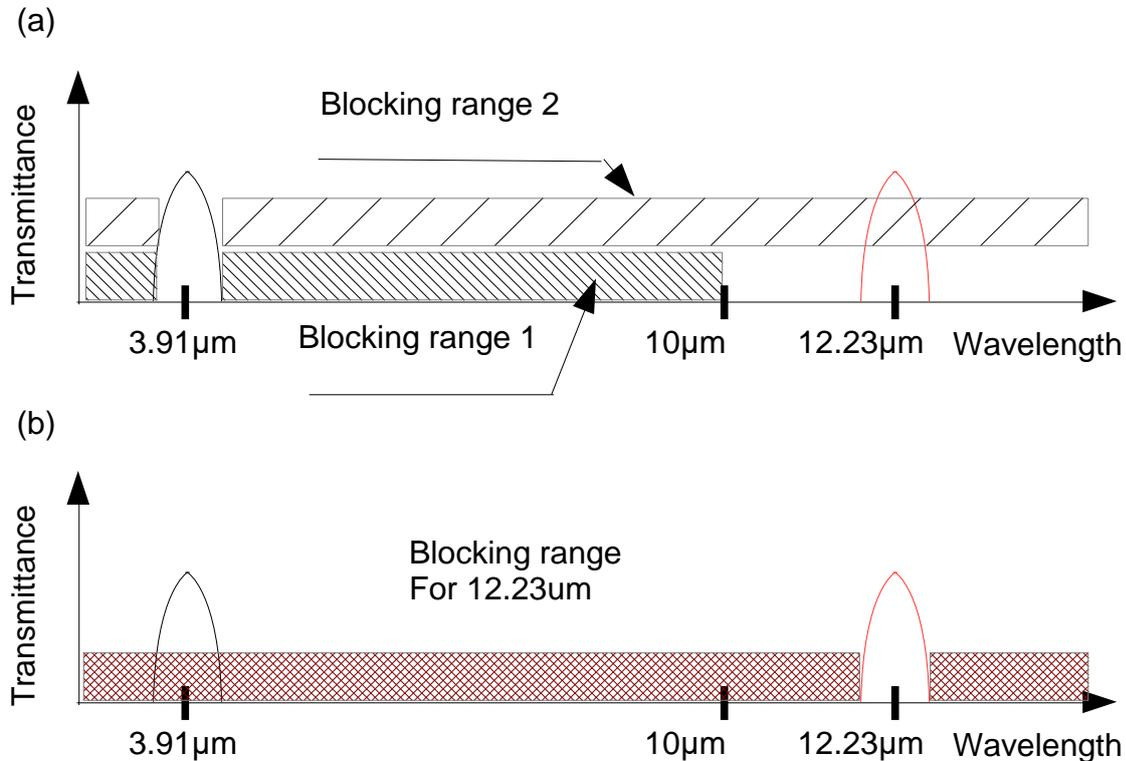
Figure 6 Simplified sketch of transmittance for both channels. (a) reference channel with two blocking ranges depending on the substrate material used, (b) signal/gas channel with its standard blocking range
