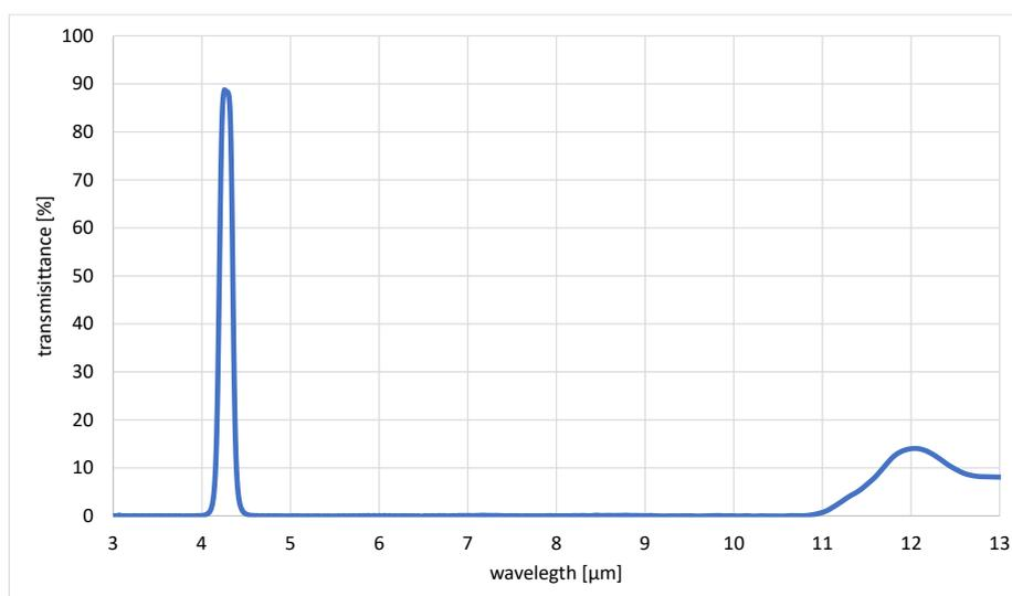
Figure 3 Filter Transmittance spectrum: 4.25 $\mu$ m CWL (central wavelength), 180nm FWHM (Full width at half maximum). Measured in an FTIR spectrometer
